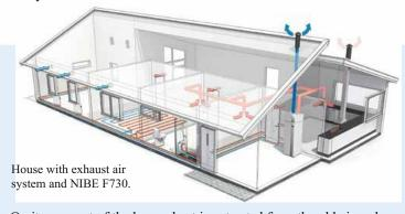
On its way out of the house, heat is extracted from the old air and transferred into the heat pump's refrigerant circuit. The cooled air is
